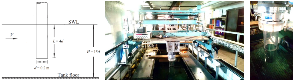
Figure 3-1 Schematics (left), PMM carriage (middle) and setup for surface piercing truncated cylinder (right)
